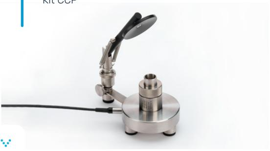
Connection: 0 V/CCP Volume: 1260 @ 500 Hz Dyn range: 25 dB(A) to 153 dB
