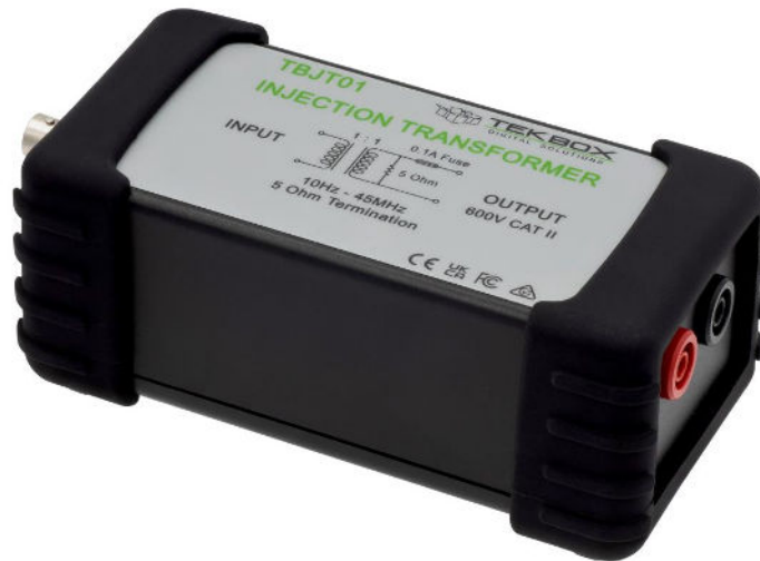
Picture 1: TBJT01 injection transformer
